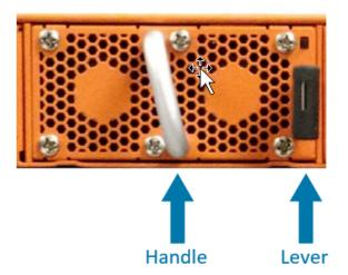
Figure 14 Replacing a Fan (GigaVUE TA Series-TA10 Shown)
