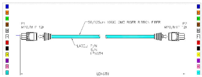
Figure 21 MPO/MTP 12 Position Fiber Cable
