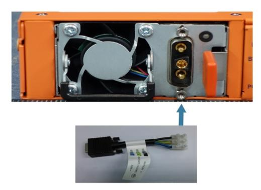
Figure 13 Connecting -48V DC Power Cable Adapter
