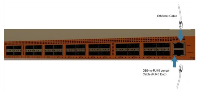
**Figure 15** Connecting the Console and Management Ports
