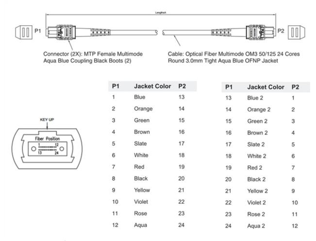
Figure 23 MPO/MTP 24 Position Fiber Cable
